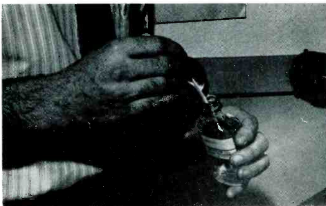
Left: Dipping a brush into a cleaning fluid is quick and easy, but unsanitary and highly undesirable since any deposit of dirt on the brush comes off and mixes with the whole bottle of fluid. Right: This illustrates the correct way to soak the brush with cleaning fluid. Here the use of an eye-dropper is made to transfer the fluid to a small nylon brush.
